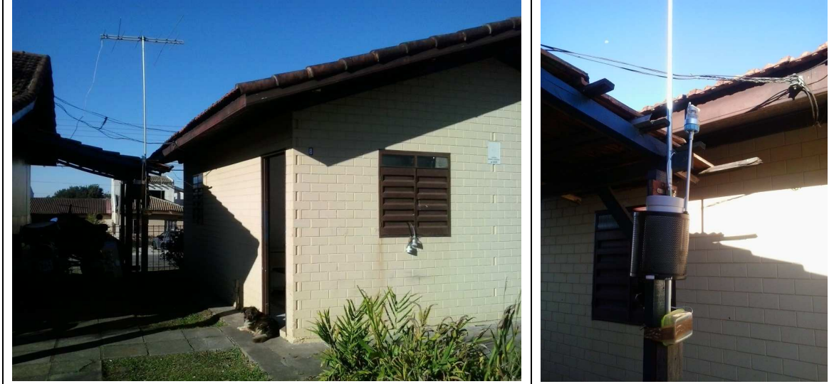
Figure A2.2. Instruments installed at Sitio Cercado, Guarda Municipal office with sampling lines of DustTrak and AE51 through the window (left) and detail of the Ecotech sampler (right).
