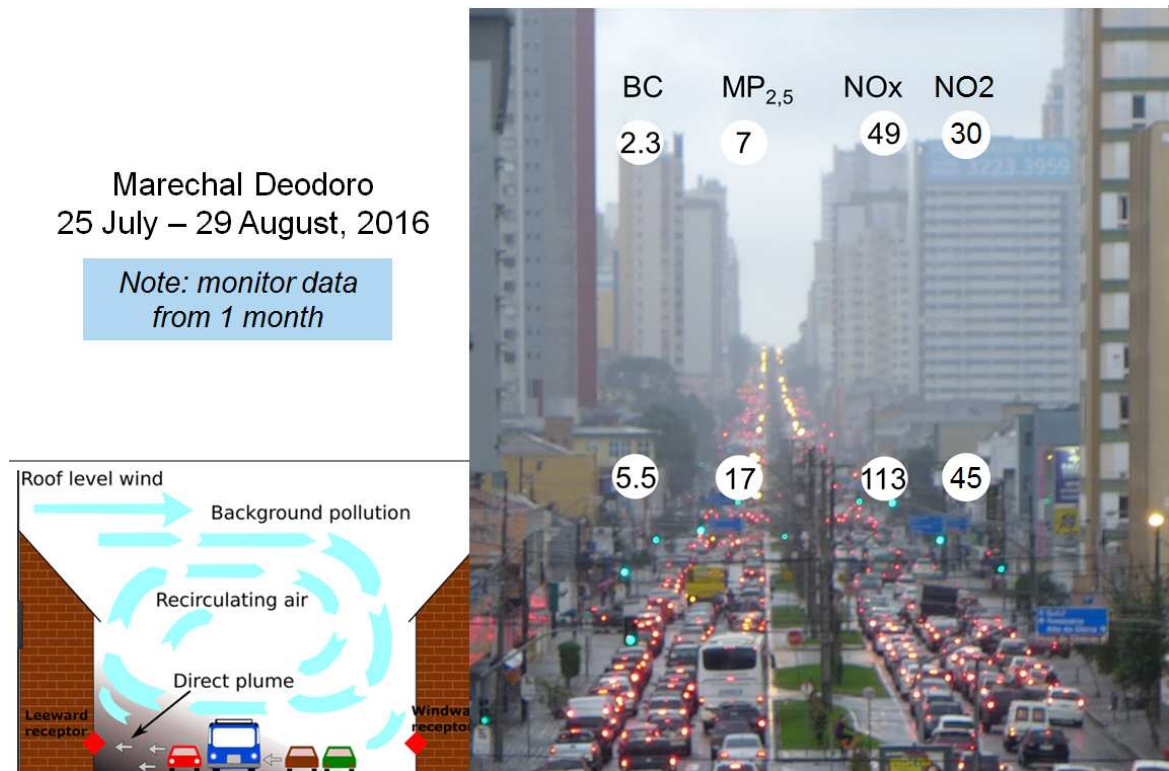
Figure ES2 Overview of how local traffic can increase air pollution levels inside a street canyon in Curitiba, adding to the urban background levels registered at roof level. Measurements made in the Marechal Deodoro street canyon. Note: The photo is from another street, used for illustrating how the buildings contribute to a canyon-like structure with reduced ventilation (also illustrated in the figure to the left).
